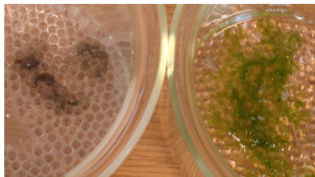
Fig. 4. Cladophora samples after 4 days of sunlight exposure (~6 h/day) with \text{TiO}_2 -covered glass beads (left) and glass beads (right) in deionized water.
